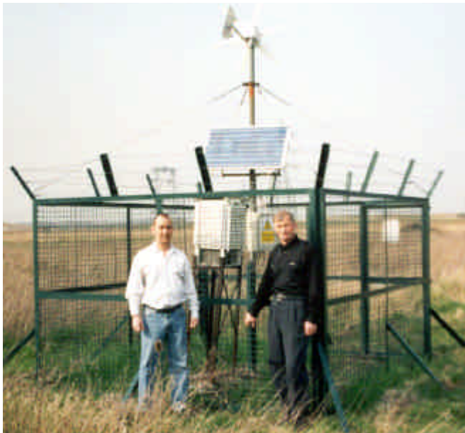
Frank Boyes, BRM (left) and Boris Popov, Baltelectro, inspect the new solar and wind powered perimeter air quality monitoring station
