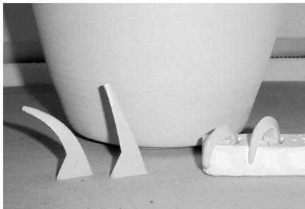
*Pyrometric cones used to measure firing heat work. Slightly slumped free-standing cones at left, Fully down plaque cones at right.*
